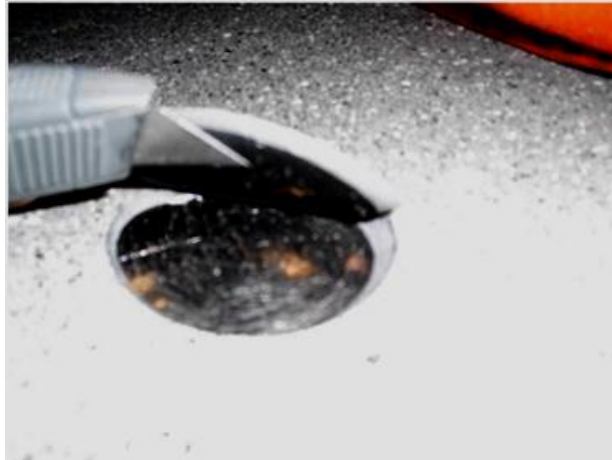
Figure 2: Delamination caused by Rust
