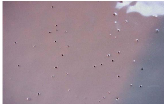
Figure 1 Ballooning and Pinholing
